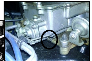
The Idle Mixture adjustments are on the bottom front of the carb
