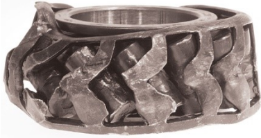
Mixing different types of grease caused this bearing to lose the lubricant and fail from excessive heat build-up from friction.
