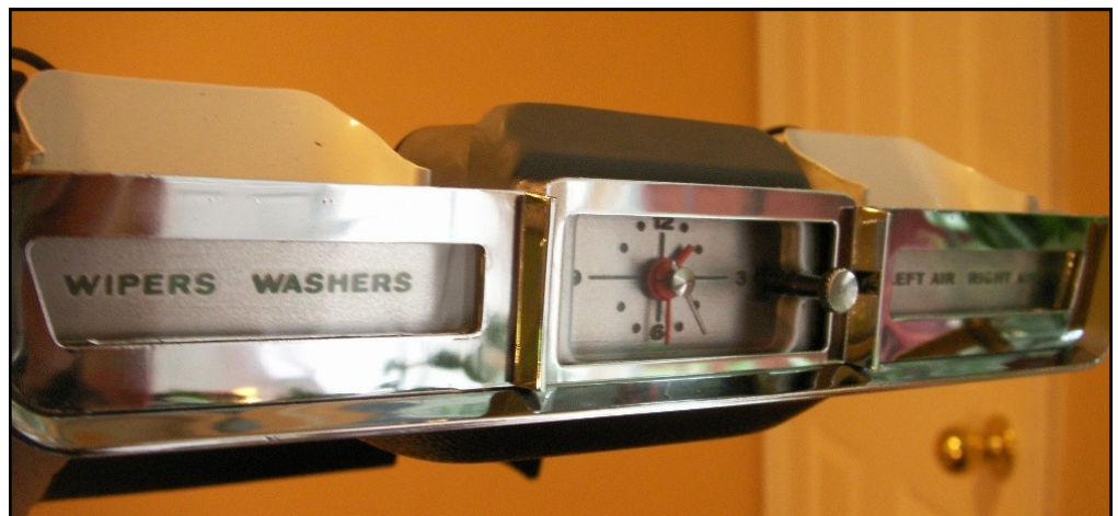
Picture 7. The completed project. Since I had the whole thing apart I repainted the black accessory cover and white reflectors behind wipers/washers/air, polished the chrome and replaced the other two clear plastic faces. It is all ready to go back in the T-bird!
