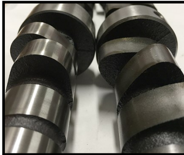
The differences in shape of a cam shaft that uses roller tappet (left) and flat tappet (right) lifters.
